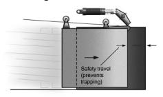
The fire door travels quickly until it reaches the lever. It is then gently decelerated by the lever mounted shock absorber and closes without shock or danger to personnel.
