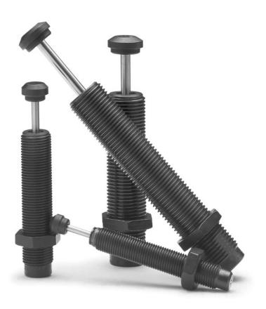
SC<sup>2</sup> Series Miniature Shock Absorbers provide dual performance benefits. They offer soft contact deceleration where initial impact reaction forces are very low, with the advantages of self-compensation to react to changing energy conditions, without adjustment. They have long stroke lengths, SC<sup>2</sup> 925 with 1.58 inch (40 mm) superstroke, to provide smooth deceleration and low reaction forces.
