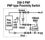
Supply Voltage: 10 to 27 VDC Ripple p to p 10% max
