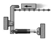
By means of a lever the effective stroke length can be increased and mounting space to the left reduced.
