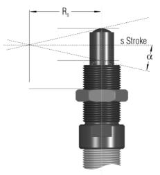
Problem: Rotary motion of the striking surface creates side load, which develops a bending moment on the piston rod. This can bend the rod in some cases. In all cases, side
