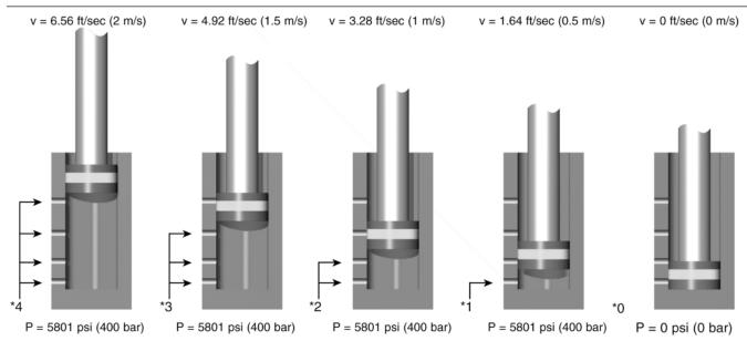
\* As a moving load impacts the shock absorber, the piston travels through stroke and forces hydraulic fluid through the multi-orifice inner tube. The total orifice area decreases at a rate consistent with the decay of impact velocity, resulting in true linear deceleration.
