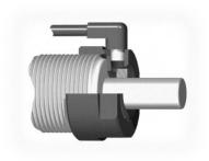
By using this air bleed collar the operating lifetime of shock absorbers in aggressive environments can be considerably increased. The adapter protects the shock absorber seals from cutting fluids, cleaning agents, cooking oils etc. by using a low pressure air bleed.
