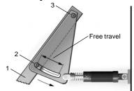
The lever 1 swings with the pin 2 in a slotted hole around pivot point 3. The lever is smoothly decelerated at the extreme end of its travel.
